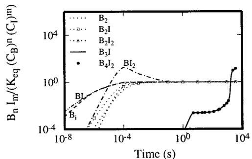
FIG. 2. Simulations using the full cluster model of normalized cluster concentrations (relative to their equilibrium value) versus time for an 800 °C anneal. Note that the curves for B<sub>3</sub>I and B<sub>4</sub>I<sub>2</sub> overlap.
