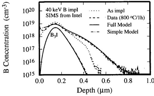
FIG. 4. Comparison of full model with the simplified model for a 40 keV  $2 \times 10^{14} \text{ cm}^{-2}$  B implant annealed at 800 °C for 1 h. Also shown for comparison are secondary ion mass spectrometry (SIMS) data from Intel (Ref. 26). Note that the full model and simple model show indistinguishable final profiles. The  $B_3I$  concentrations for the two models are also nearly identical.
