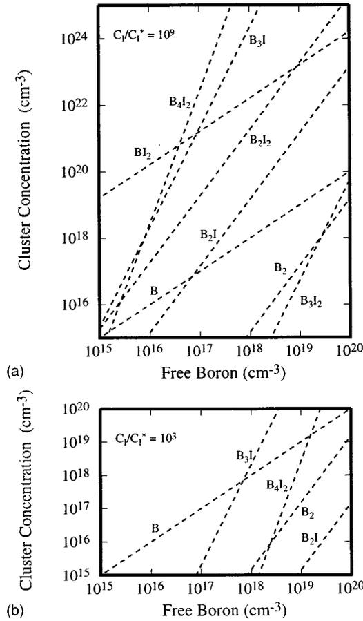
FIG. 3. Equilibrium cluster concentrations ( $K_{B_n I_m} C_B^n C_I^m$ ) vs free boron concentration at 800 °C for free interstitial concentrations of (a)  $10^9 C_I^*$  characteristic of very early stages of TED, and (b)  $10^3 C_I^*$  typical of TED conditions in the presence of {311} defects. Initially,  $BI_2$  is the primary cluster and helps immobilize the boron, while  $B_3I$  is the primary cluster during most of the anneal.
