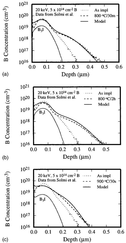
FIG. 7. Comparison of simple model to experimental data for a  $5 \times 10^{14} \text{ cm}^{-2}$  B implant annealed at (a) 800 °C for 30 min (b) 800 °C for 2 h (c) 900 °C for 30 s. SIMS data from Ref. 12.
