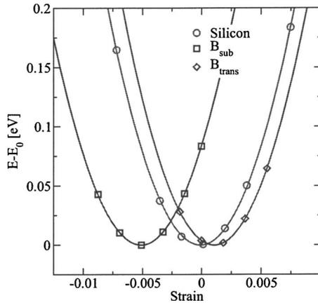
FIG. 2. Energy vs hydrostatic strain for Si, substitutional B, and BI transition state ( $B_{\text{trans}}$ ) under hydrostatic strain. Strains are reported in reference to the GGA Si equilibrium lattice parameter. Energies are plotted relative to the minimum energy for given configuration,  $E_0$ .
