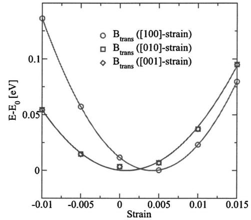
FIG. 4. Energy vs uniaxial strain in different directions for the transition state of  $BI_{\text{tet}} \rightarrow BI_{\text{hex}}$  with hop vector  $(3,1,1)b/8$ , where  $b$  is the Si lattice constant. Note that the strain effect is largest in the dominant direction of motion.
