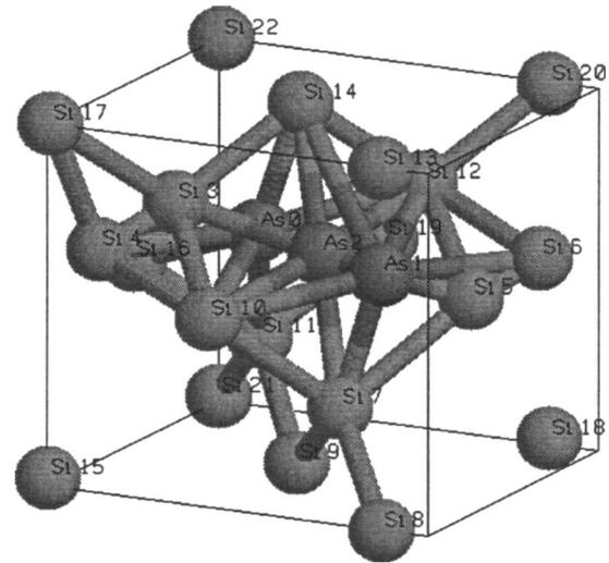
FIG. 6. Three-dimensional view of  $AsI_{(110)\text{split}} \rightarrow AsI_{\text{hex}} \rightarrow AsI_{(110)\text{split}}$ . As migrates from a split position (As0 site) to another split position (As1 site) via hex site (As2 site). Si4 and As0 make (110) split for Si lattice site of Si3. Si6 and As1 also make split for Si5. As migrates from As0 to As1 position, the Si atom at Si4 site moves to original lattice point at Si3 site and Si atom at Si5 moves to Si6.
