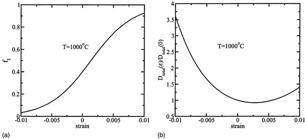
FIG. 9. Strain dependence of (a) fractional contribution to As diffusion by interstitial mechanism ( $f_I$ ) and (b) total As diffusivity normalized to unstrained value. Diffusion mechanism changes from vacancy mediated to interstitial mediated in going from compressive to tensile strain.
