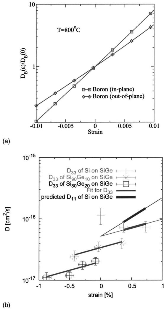
FIG. 5. B diffusion enhancement as a function of biaxial strain at  $800^\circ\text{C}$  from (a) predictions based on DFT calculations, and (b) experimental data by Kuo *et al.* (see Ref. 16). The vertical B diffusion enhancement was measured under biaxial strain using SiGe bilayers with different Ge content (blue lines fitting data). The data were combined with hydrostatic B diffusion data from Aziz *et al.* (see Ref. 17) to estimate the lateral B diffusion enhancement (upper black line).
