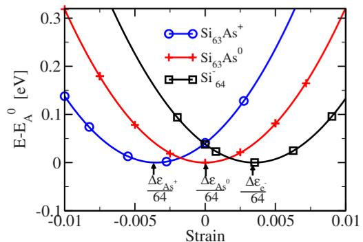
FIG. 1. (Color online) Energy vs hydrostatic strain curve for 64 atom supercell with  $\text{As}^+$ ,  $\text{As}^0$ , and  $e^-$ . The normalized induced strain is defined as  $\Delta\epsilon = 64 \times (a - a_0)/a_0$ , where  $a$  is the equilibrium lattice constant of the supercell with a dopant or an electron and  $a_0$  is the Si lattice constant.
