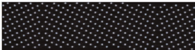
Figure 5 (online colour at: www.pss-b.com ) System used for validation of MS model. Two twin grain boundaries are separated by an ideal (ballistic) crystalline region.
